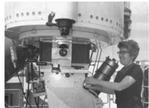
Vera Rubin operated the 2.1-meter telescope at Kitt Peak National Observatory, Kent Ford's spectrograph is attached to the telescope.
